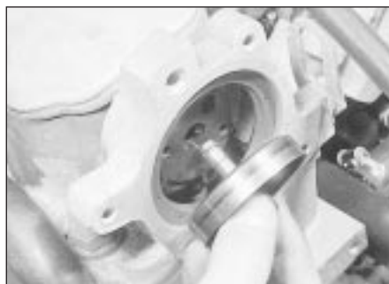
3.11a Extract the rotor hub . . .
